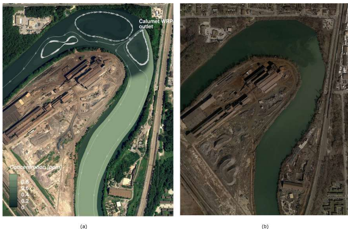
Fig. 8. Tracer simulation near the outflow of the Calumet WRP. The Left figure is the simulation result. The right figure is an aerial image from Google Earth.
