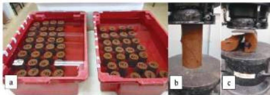
Figure 11. Preparation of specimens for UCS and STS tests a) submersion of specimens; b) UCS test; c) STS test.
