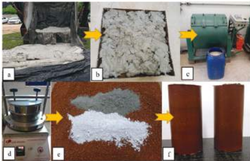
Figure 6. Preparation of the waste glass powder a) waste glass (sludge); b) drying c) fragmentation; d) sieving; e) blend composed by soil, PC, and WGP; f) moulded specimens with soil, PC, and WGP.
