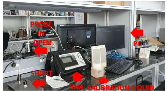
Fig. 2. Setup for measurement of dielectric properties
