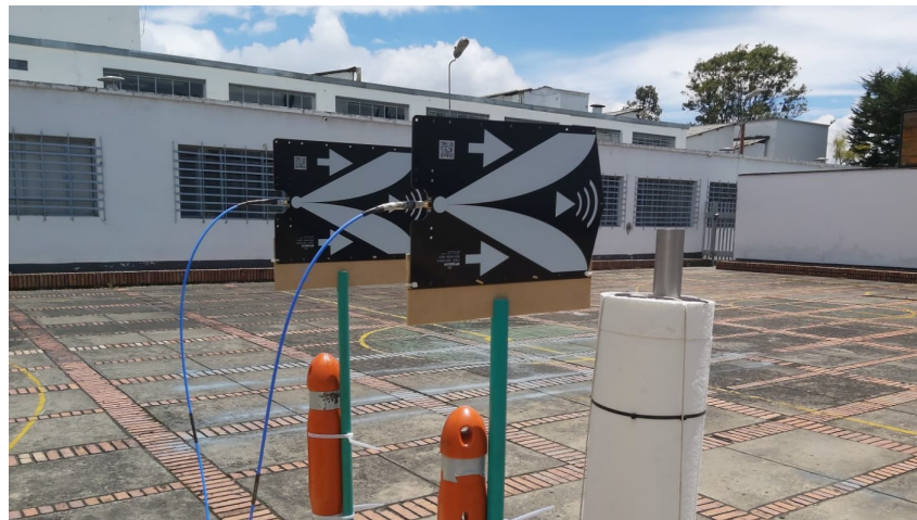
Figure 15. Experimental setup for free space experiments and the metal cylinder with two Vivaldi antennas.
