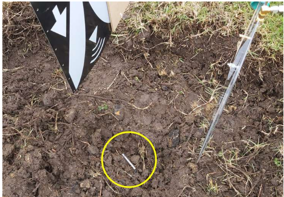
Figure 9. Buried objects experimental setup with a metal IED detonator.
