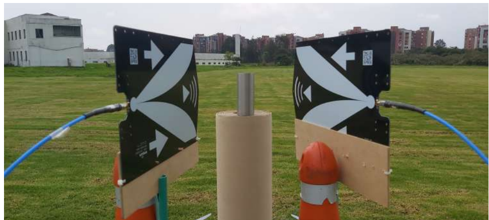
Figure 5. Free space experimental setup with a metal cylinder.
