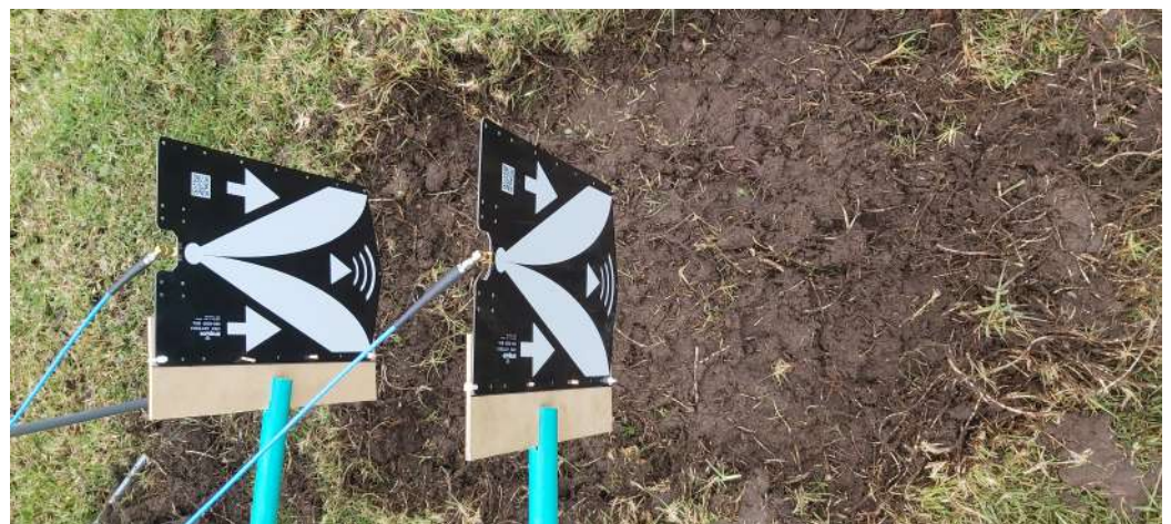
Figure 8. Buried objects experimental setup, soil alone.
