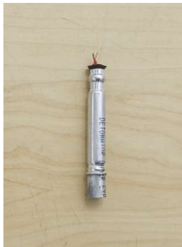
Figure 5-10.: Electric IED detonator commonly used in Colombia. The approximate dimension is 54 mm with a diameter of 4 mm.
