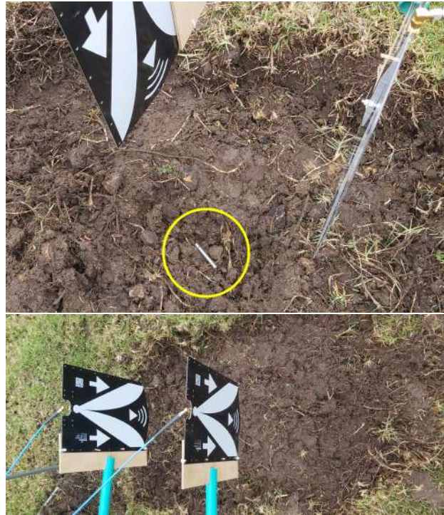
Figure 5-9.: Buried metal IED detonator and Vivaldi antennas for GPR measurements.
