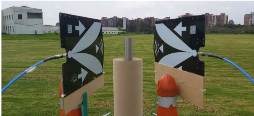
Figure 5-5.: Metal cylinder for free space experimental setup in frequency domain CNR calculations.
