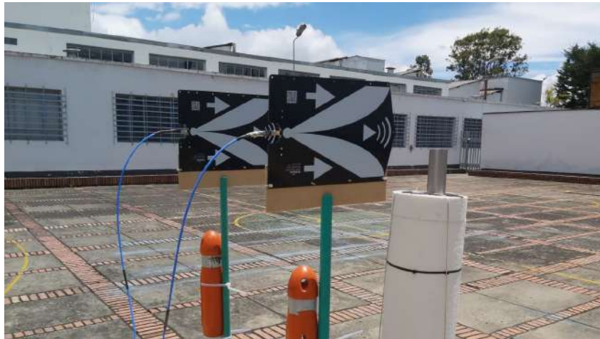
Figure 3-11 .: Basic setup for a metal cylinder backscattering scenario in free space.
