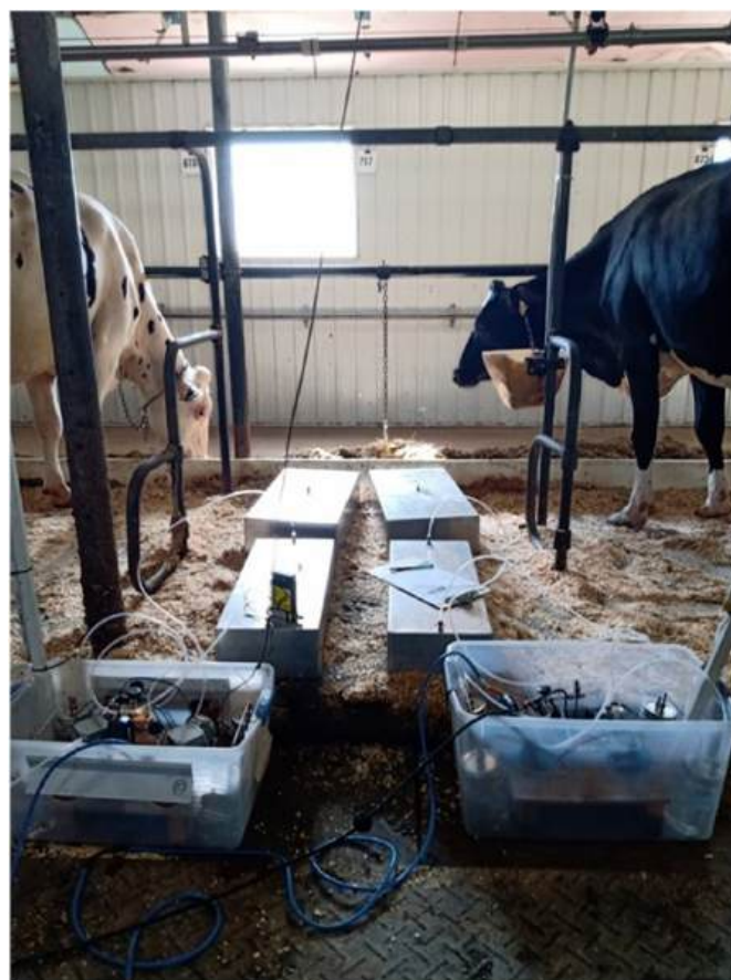
Fig. 2. Gas sampling is performed in closed chambers for greenhouse gases (four boxes in the back) and by the bubbling method for ammonia (two containers in the front) in tie-stalls.
