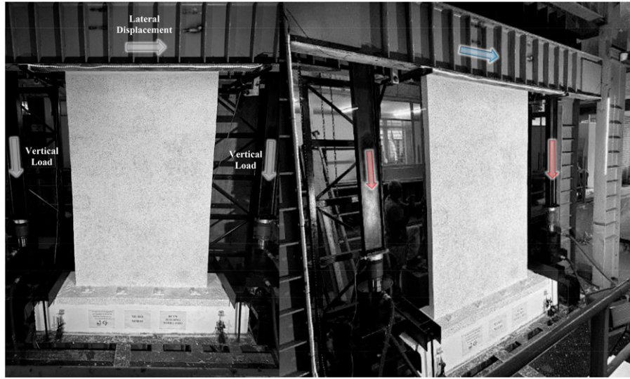
Figure 5. The experimental assembly of the TRCW-M3R10 specimen on the THF.
