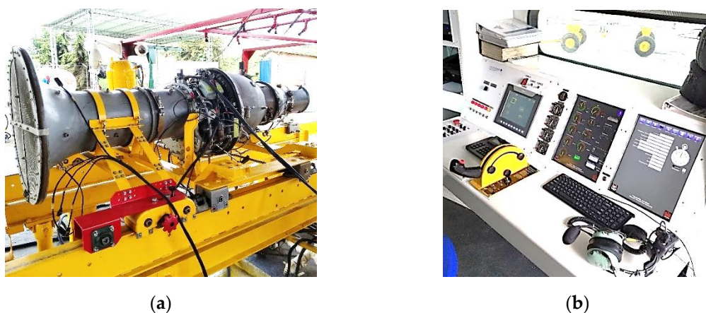
Figure 1. (a) General aspect of the J69 engine installed in the testing bench; (b) detail of the control booth used in the experimentation.
