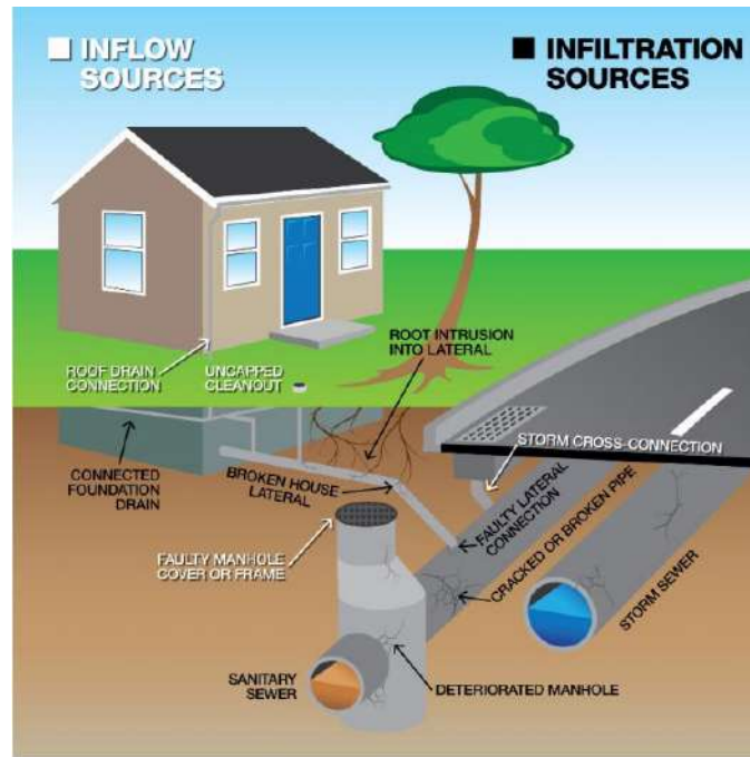
Figure 2.1. Typical Sources of I/I in sanitary sewer systems (WEF, 2017)
