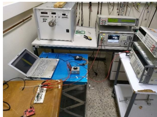
Figure 4. Left: Circuit connection for calibration of high accuracy current sources using a current switch. Right: Experimental setup to test the current switch system using a 100 \Omega resistor.
