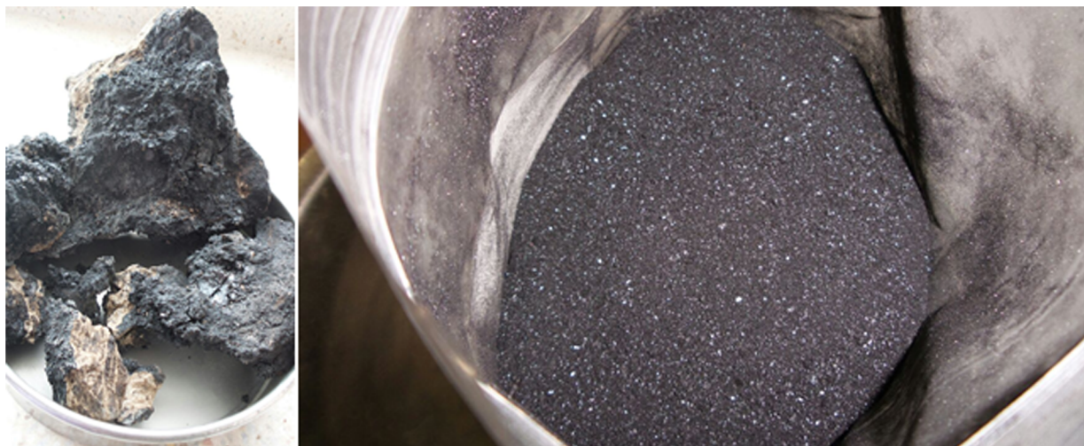
Fig. 1. Gilsonite before and after milling (images by Hugo Alexander Rondón Quintana)
