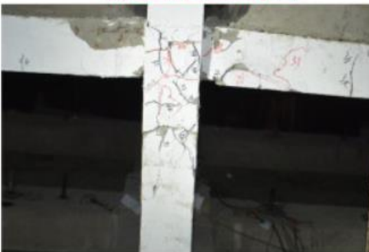
(c) Cracks of the first story after the triaxial loading under the excitation of 1.79 g
