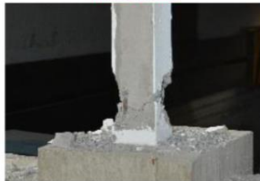
(c) Cracks of the first story after the triaxial loading under the excitation of 1.79 g
