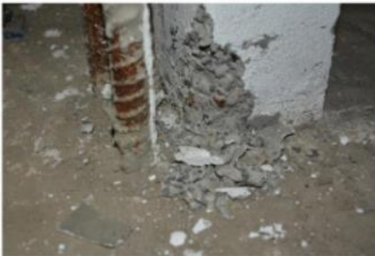
(b) Cracks of the first story after the triaxial loading under the excitation of 1.11 g
