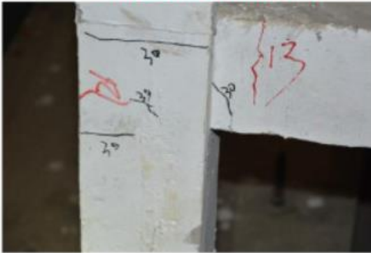
(a) Cracks of the first story after the triaxial loading under the excitation of 0.72 g
