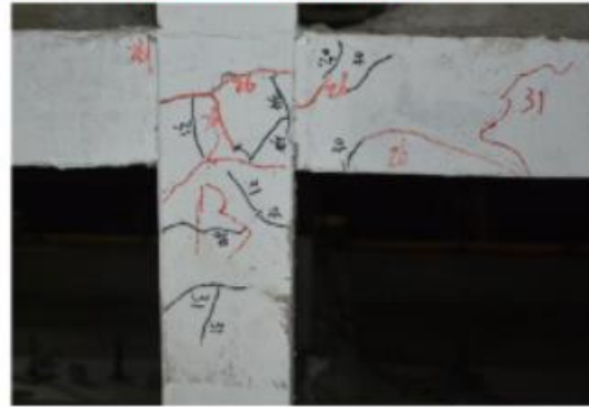
(a) Cracks of the first story after the triaxial loading under the excitation of 0.72 g
