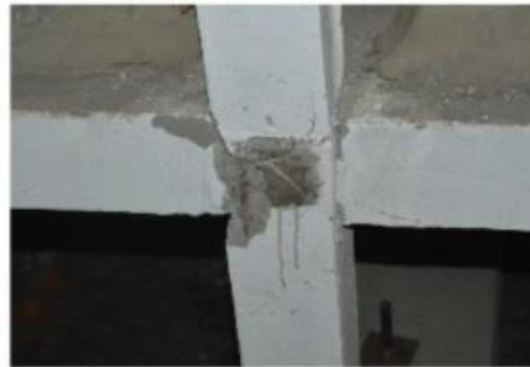
(b) Cracks of the first story after the triaxial loading under the excitation of 1.11 g
