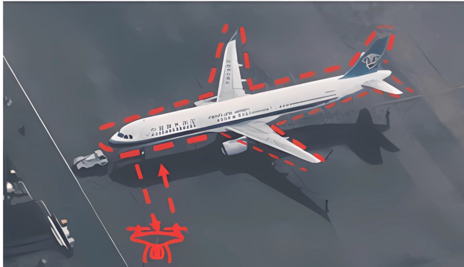
Fig. 7. Drone inspection trajectory for an aircraft, source: Authors.
