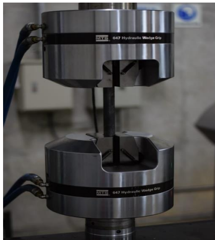
Figure 1. 810 material test system used for tensile essay.
