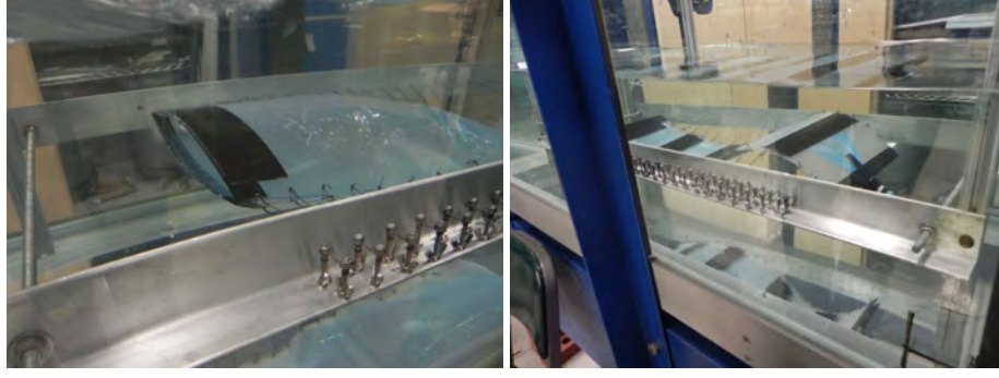
Figure 3.2: Deformed non-reinforced ribbon ( left ), and reinforced with thin stainless steel strips ( right ).
