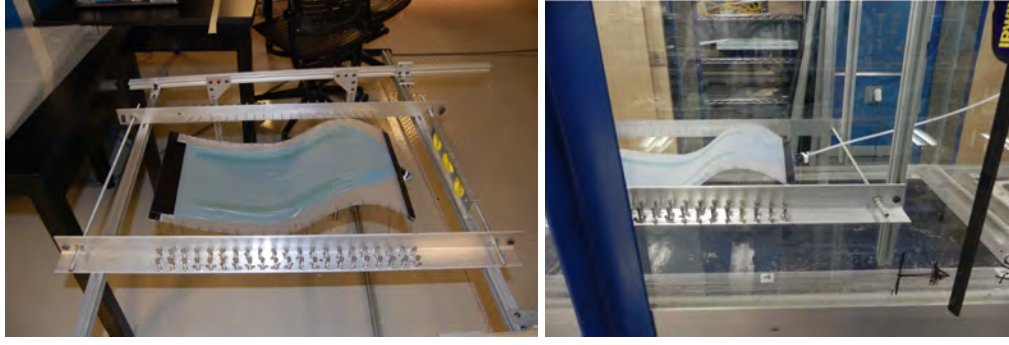
Figure 3.1: Ribbon pump, series T01 . Top view ( left ) and side view mounted on the frame suspended on top of the flume ( right ).
