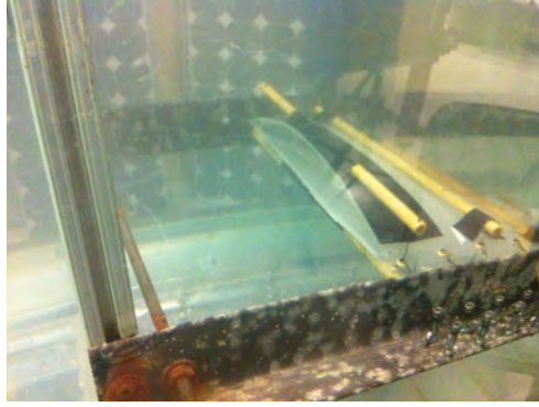
Figure 4.12: Constriction at the entrance sides due to the tension on the strings and bulging at the center on Prototype 2.4.
