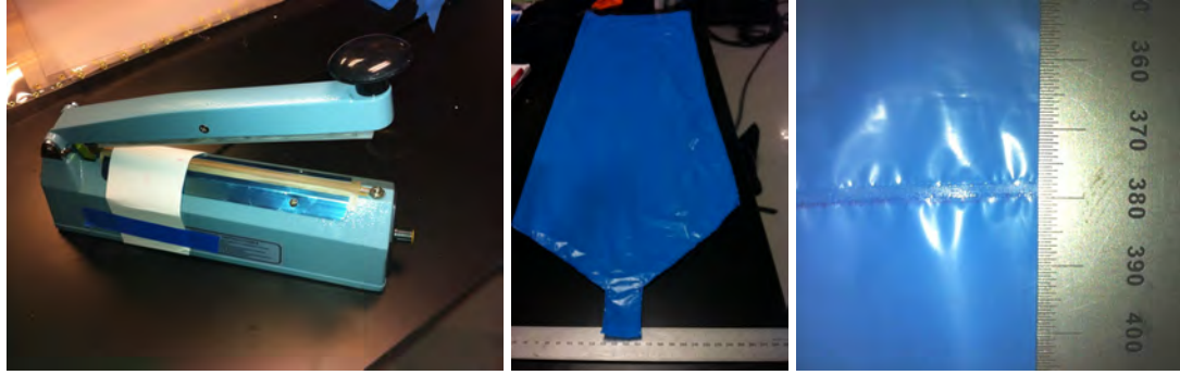
Figure 3.18: Internal membrane configuration for prototype 3: 20cm long impulse sealer ( left ); general aspect of the internal membrane, showing 10cm extension after the ribbon ends ( middle ); close-up to the 3mm seal ( right ).
