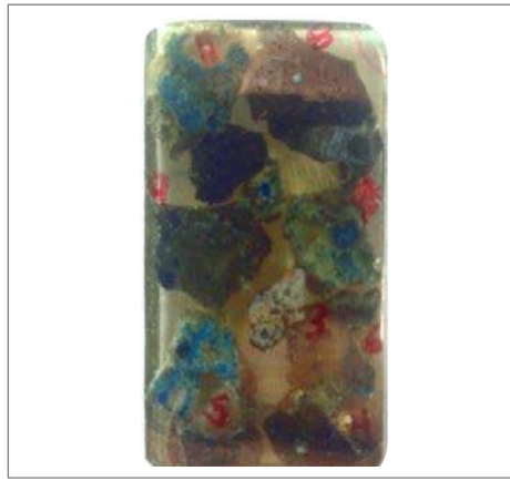
Figure 3. Sample assembled with selected grains of BFS
