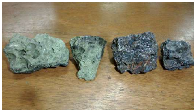
Fig. 1. Slag particles (size between 19 and 25.4 mm diameter). (Images by authors.)
