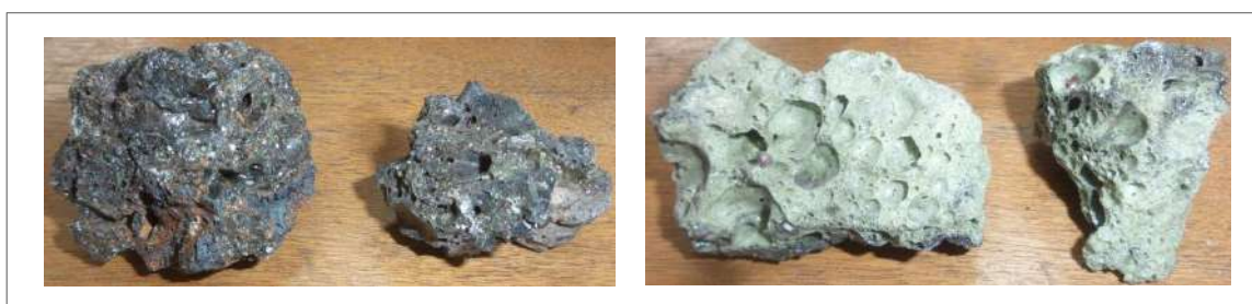
Figure 2. Slag particles (size between 3/4" and 1" in diameter)
