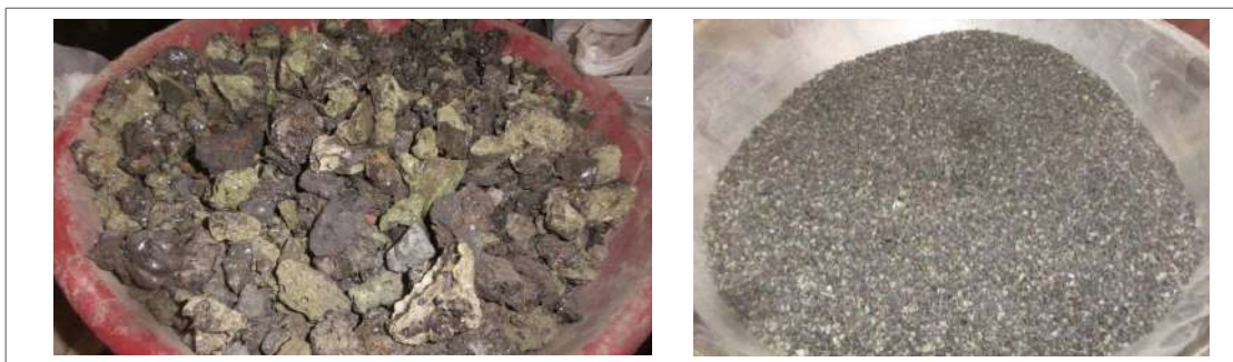
Figure 1. Slag particles (coarse and fine)
