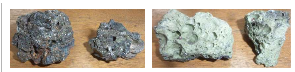
Figure 2. Slag particles (size between 3/4" and 1" in diameter)
