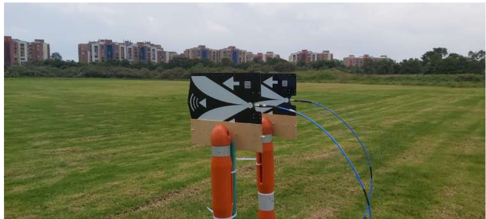
Figure 4. Free space experimental setup with no objects.
