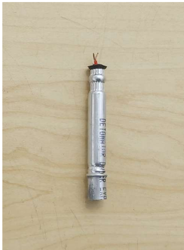
Figure 10. Electric IED detonators commonly used in Colombia. The approximate dimension is 54 mm, with a diameter of 4 mm.
