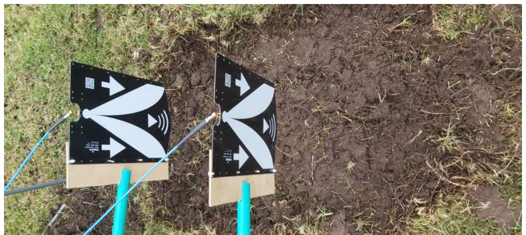
Figure 8. Buried objects experimental setup, soil alone.
