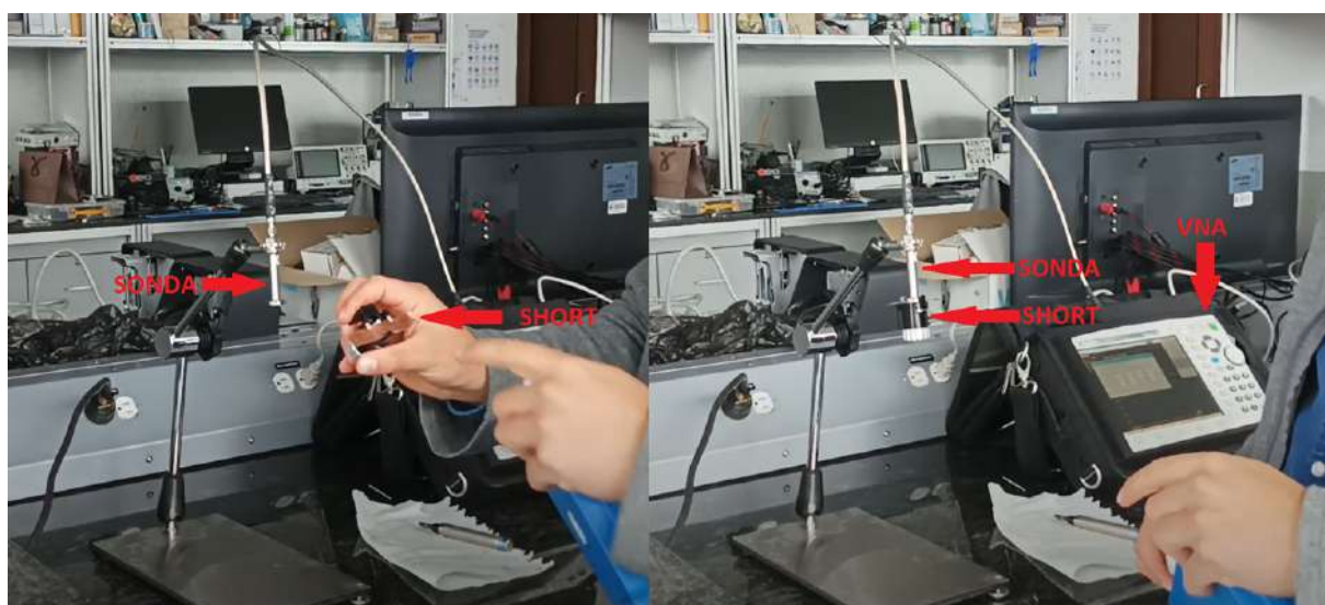
Figure 1.5: Set measurement system calibration (VNA - Probe) short circuit (Short)
