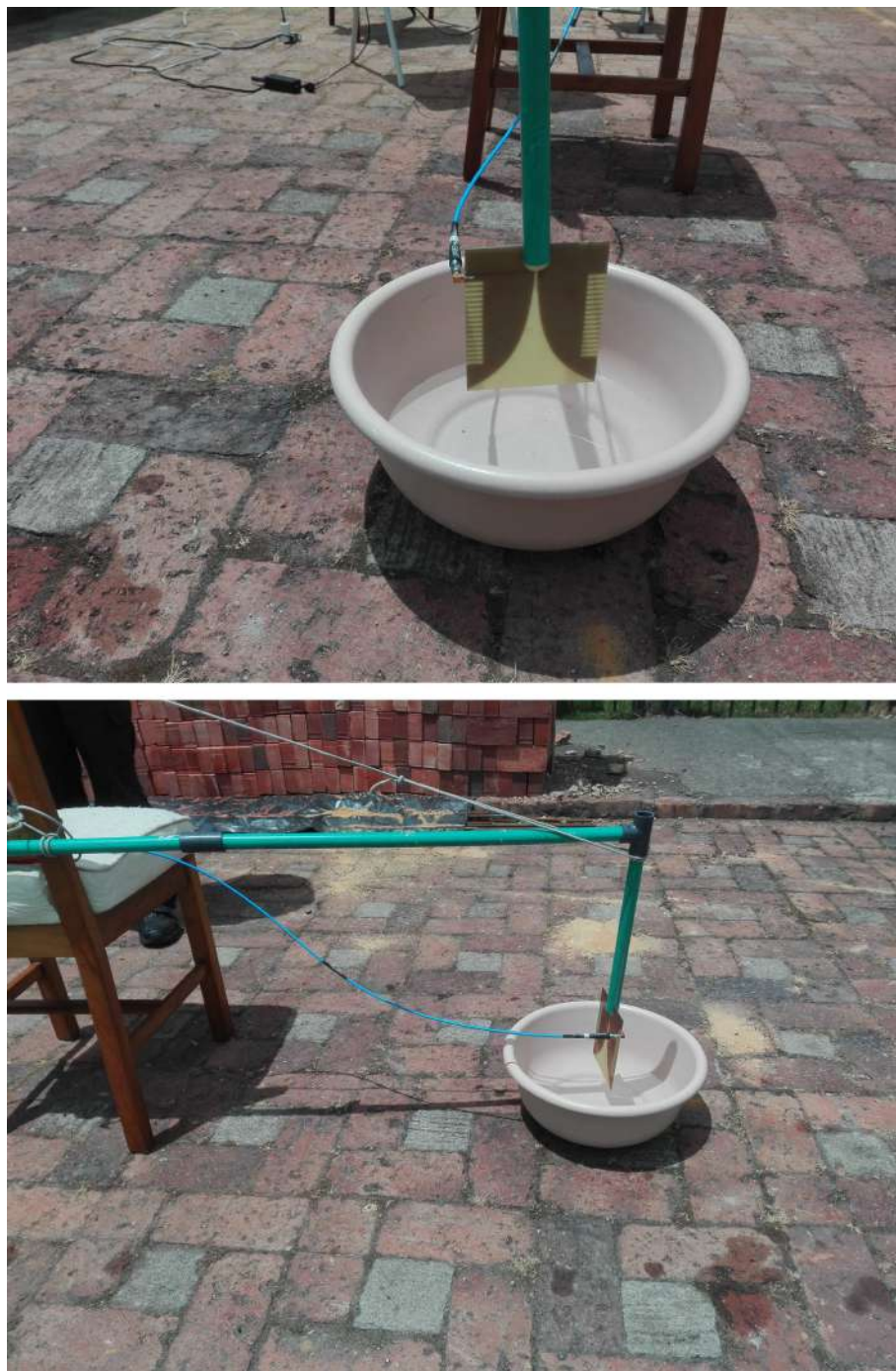
Figure 3.11: Electrical permittivity measurement set up of water in Bogotá, Colombia
