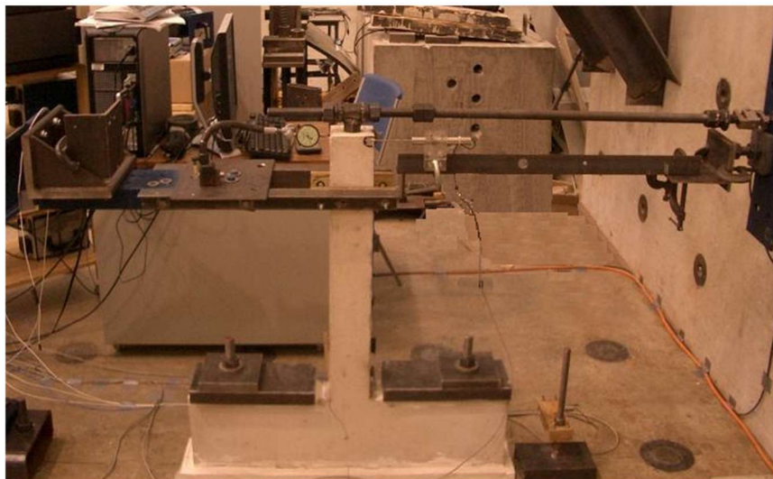
Figure E-5 Set-up of pseudo-static tests of small-scale specimens.
