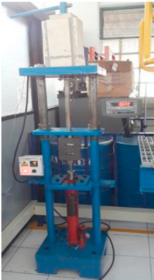
Figure 2. Briquetting press developed for the current investigation. Source: Authors.
