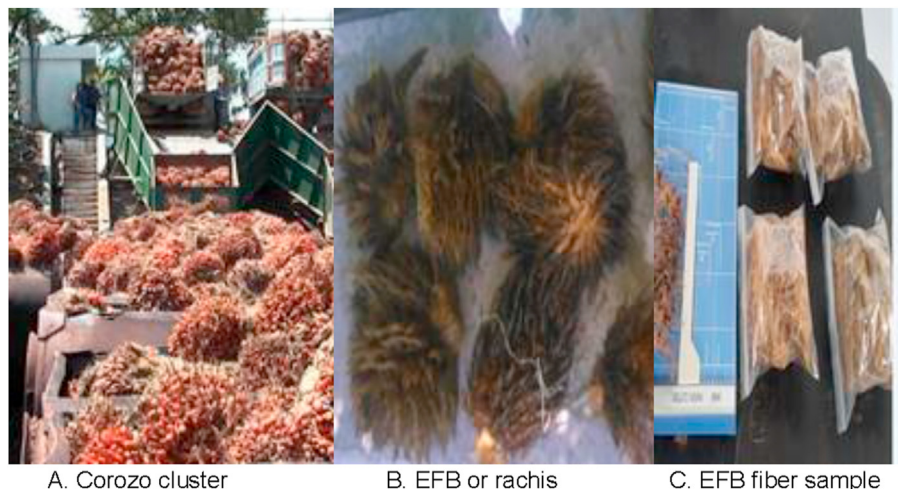
Figure 1. Raw material states from corozo to storage of cut fiber in airtight packages. Source: Authors.
