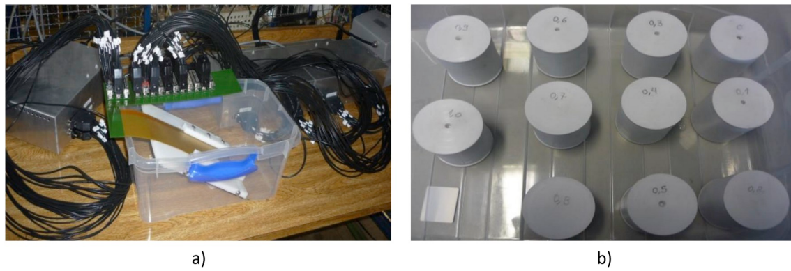
Fig. 9. Calibration elements. a) Calibration box and b) Sample of cylinders.
