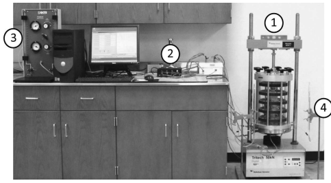
Figure 3. Servo/suction-controlled plane strain testing system.
