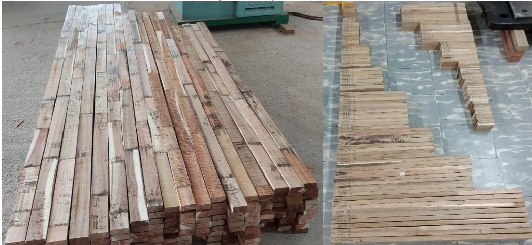
(a) Sheets obtained from the manufacturing process. (b) Tested specimens, only one group. Source: Authors' own work.
