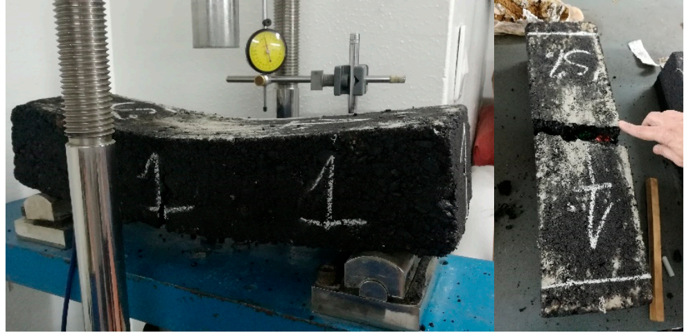
Figure 9. Deformation of the beam at the end of the test.
