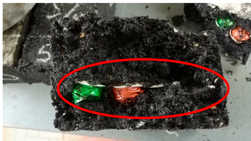
Figure 8. Position of the capsules in the lower third of the specimen after failure.
