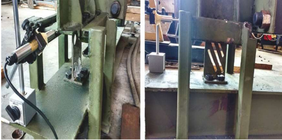
Fig. 3. Examples of an experimental test of the SSD dampers.
