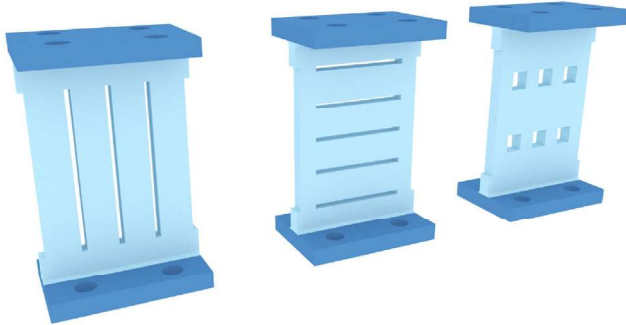
Fig. 6. Examples of slotted damper.
