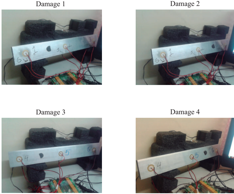
FIGURE 2.12: Aluminum rectangular profile instrumented with 6 piezoelectric sensors.
