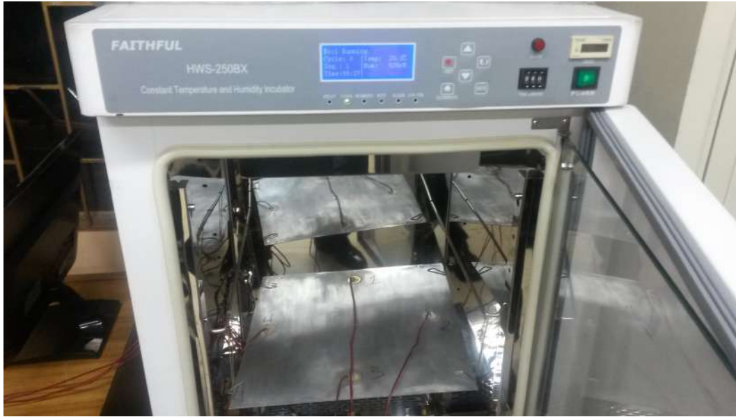
FIGURE 3.9: Aluminum plate inside the climate chamber (Faithful HWS-250BX).
