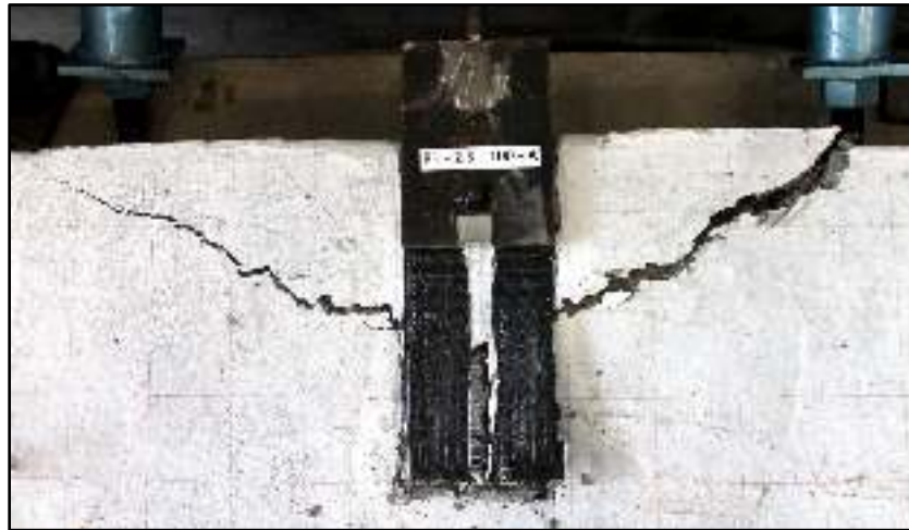
Figure 74 Crack formation in specimen R1 – 2.5 – 100 – A . Source: Own.
