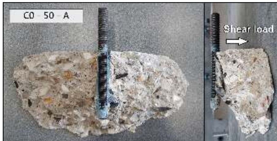
Figure 29 Concrete breakout body C0 – 50 – A. Source: Own.
