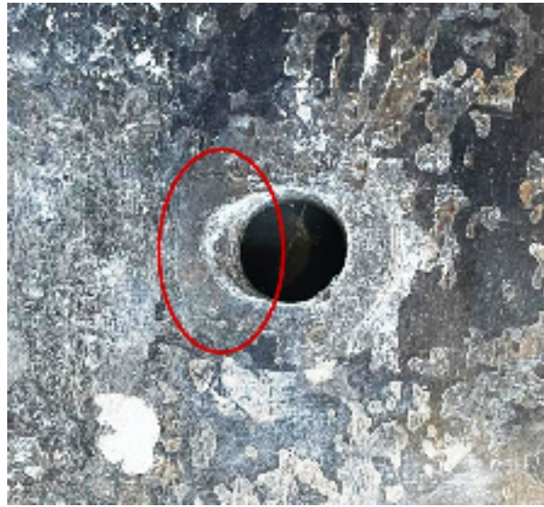
Figure 76 Wear on the steel plate due to accumulated tests. Source: Own.
