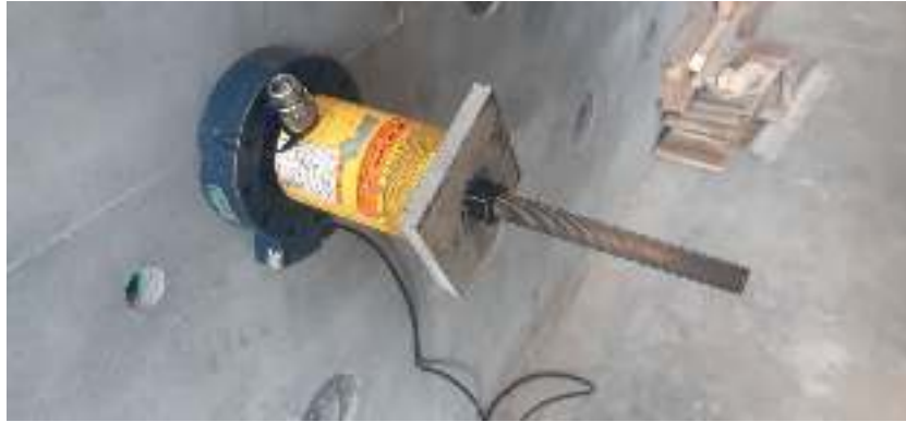
Figure 19 Hydraulic jack used for testing. Source: Own.
