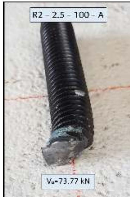
Figure 64 Anchor failure R2 – 2.5 – 100 – A. Source: Own.
