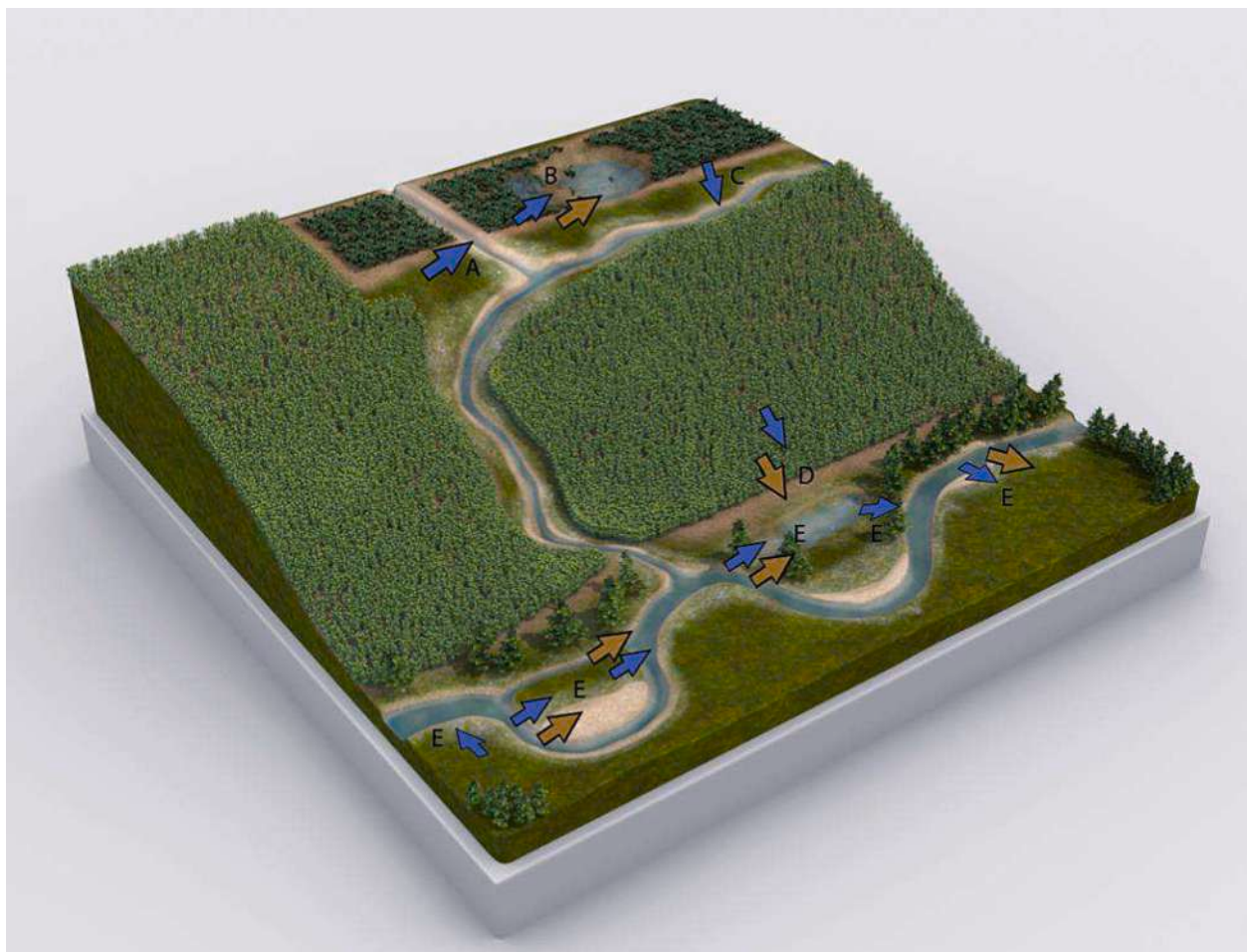
Fig. 4. Connectivity of landscape elements in the Upper Sangamon River Basin. Block diagram is vertically exaggerated to emphasize landscape position. Uplands are low-relief and occupied by intensive agriculture (upper portion of block diagram). The floodplain is situated within a broad valley created by glacial meltwater. Connectivity of water (blue arrows) and sediment (brown arrows) varies within the landscape. In the uplands, drainage ditches (arrow A) and small tributaries (arrow C) receive water from uplands via tile drains, grassed waterways, groundwater and limited overland flow. Closed depressions (arrows at B) are common on the landscape and trap water and sediment. Bank erosion occurs in tributaries, producing sediment, but much of the sediment eroded on the uplands is transported short distances and redeposited with limited connectivity to ditches or tributary streams. Transport on hillslopes along valley bluffs (arrows at D) move water and sediment to the edge of the floodplain on the valley bottom. Within the floodplain (arrows at E) there is exchange of water and sediment between the floodplain and channel mediated by the morphology of the channel banks and the adjacent floodplain. Image Credit: Alex Jerez, ITG, Beckman Institute. (For interpretation of the references to colour in this figure legend, the reader is referred to the web version of this article.)
