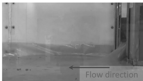
Figure 8a. Tailings flow experiment: photo and video screenshot of the experiment.
