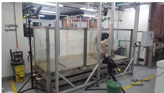
Fig. 3 Environmental flume for liquefied-tailings-flow experiments
