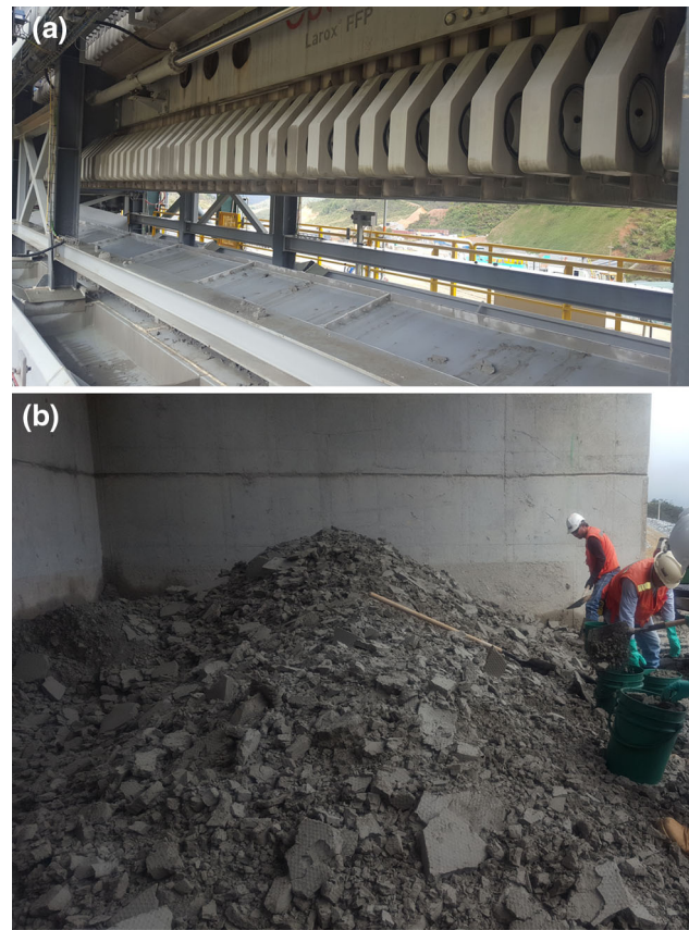
Fig. 1 Filtered tailings used in this study. a Tailings dewatering system: compressing plates with cloth filters and air injection; b pile of low water-content tailings cake produced by the tailings dewatering system
