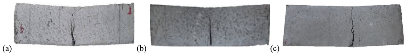
Fig. 7 Typical failure modes of beams tested under bending: a PC, b D_f = 32.0 \text{ kg/m}^3 , c D_f = 58.1 \text{ kg/m}^3
