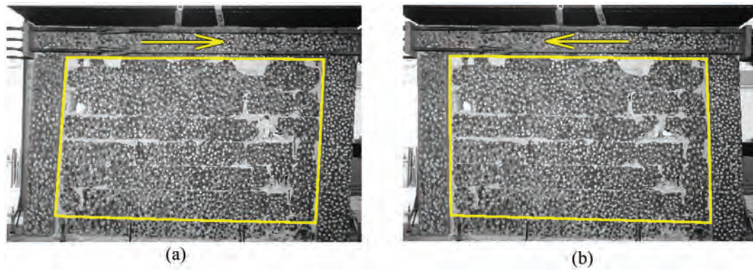
Figure 8. Images #67 and #70 of two deformed states that were used in the mesh adaption scheme (Figure 4(b)), respectively, for the most loaded state with positive (a) or negative (b) displacements in the x -direction.
