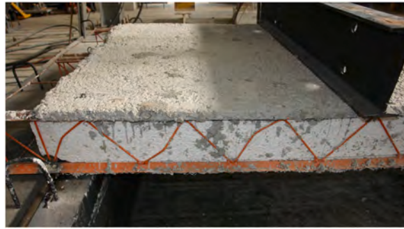
Fig. 9. Buckling of diagonals of ribs in LT1 and LT4 slab panels.
