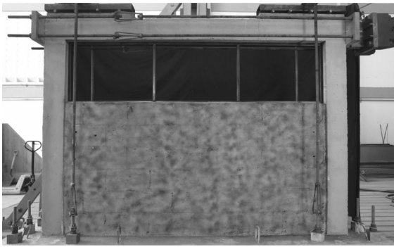
Fig. 8 Single bay partially infilled frame (PF)
