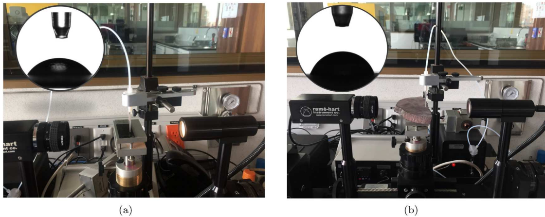
Figure 7. Contact angle for CRA and HRA Residual Asphalts under study. (a) Contact angle of CRA Residual Asphalt and (b) Contact angle of HRA Residual Asphalt.
