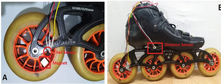
Fig. 2. Mount sensors on the skate.
