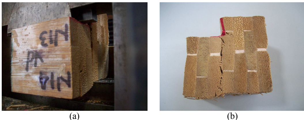
Fig. 4 – Test of shear parallel to glue line: (a) Before mechanical test; (b) Typical failure
