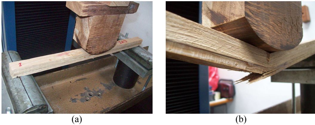
Fig. 2 – Bending test: (a) Before mechanical test; (b) Typical failure
