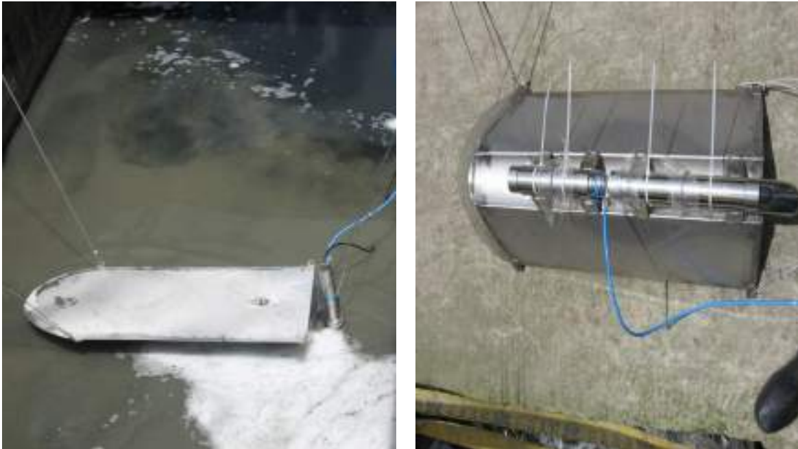
Figure 3.21 Installation boat for infra-red, ion sensitive and UV-VIS spectrometry sensors
