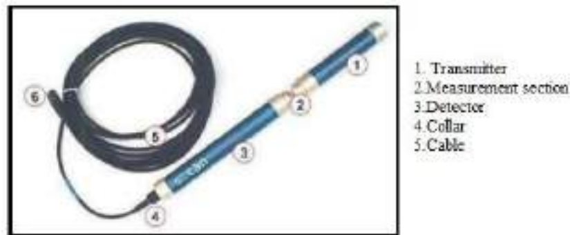
Figure 3.13 Sensor's components (s::can, 2007)
