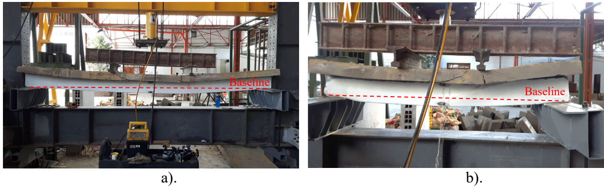
Figure 3. Final condition of specimens in full-scale beam test. a). 4m-long beams. b). 2m-long beams.
