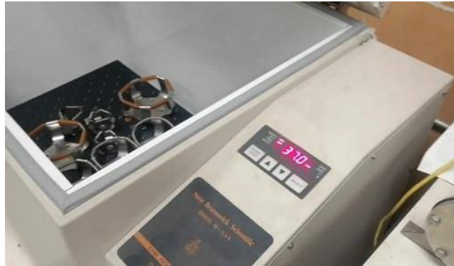
Figure 6.18. C25KC classic incubator used for placed the plates at 37°C for 24-48 hours
